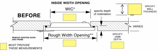
\*WIC - Width in clear from inside chamber \*\*Rough Width Opening - Width of opening from outside of chamber It is critical that we get the opening size (interior, exterior and wall thickness), not just door measurements.
