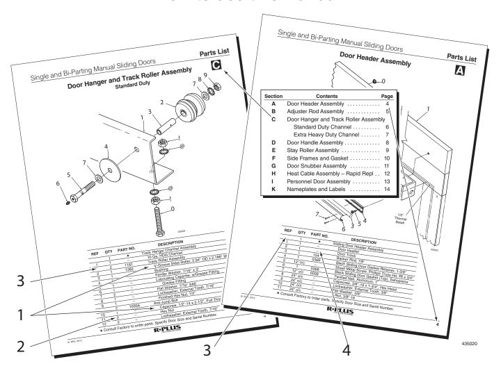
Use the front cover illustration as a guide to the sections contained in the parts manual.
