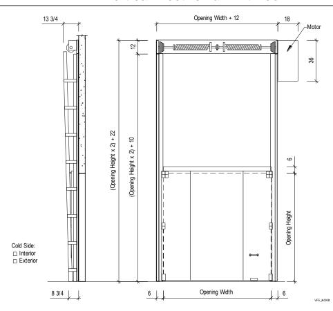
Notes: Standard slide lock included (field installed). If door is mounted on outside of room, then an alternate safety exit is required. Power cut-off switch provided on electric doors.
