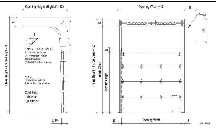
Notes: Standard slide lock included (field installed). If door is mounted on outside of room, then an alternate safety exit is required. Power cut-off switch provided on electric doors.
